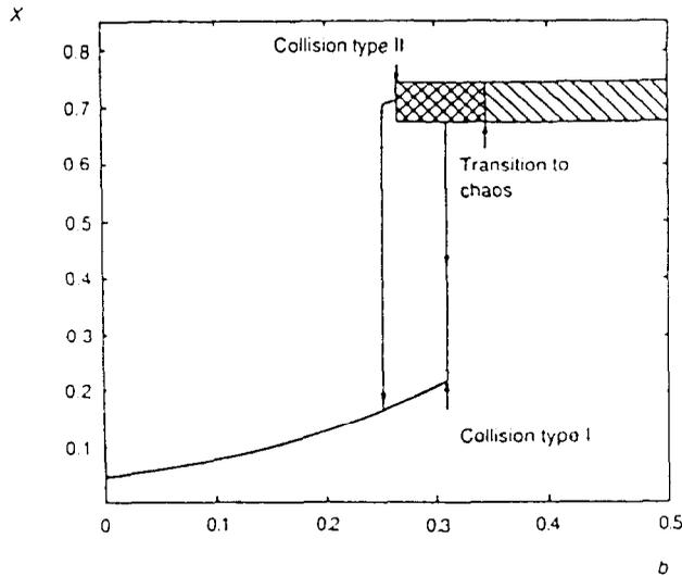
Fig. 11. Maximum deflection  $X$  vs amplitude of excitation  $b$  for equation (3.1); the 'hatching' indicates strange nonchaotic transient behaviour, and the 'cross-hatching' chaotic behaviour.
