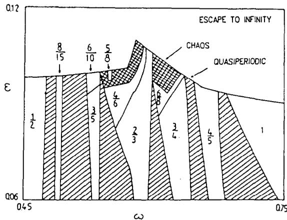
Fig. 7. Domains of chaotic (cross-hatched) and quasiperiodic behaviour of equation (2.8);  $\mu_0 = 0.95$ ,  $\omega = 0$ .
