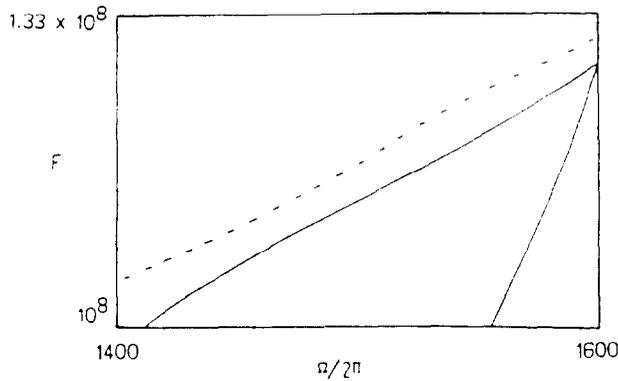
Fig. 13. Boundary of existence of the solution (2.2) (broken line) and boundaries of Hopf bifurcation (solid line) for equation (2.1). (system parameters as in Fig. 1).
