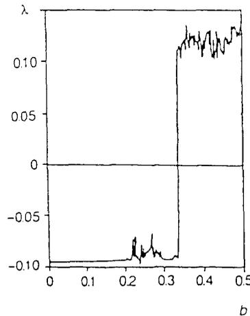
Fig. 8. The largest nonzero Lyapunov exponent  $\lambda$  vs amplitude of the parametrical excitation  $b$  for equation (3.1).
