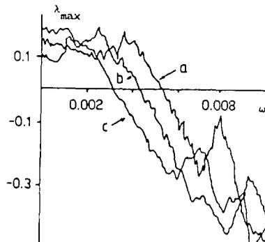
Fig. 4. The largest nonzero Lyapunov exponent  $\lambda_{max}$  for equations (2.3) and (2.4);  $\lambda = 2.5$ ,  $a = 5$ ,  $\Omega = 2.64$ ; (a) two frequency forcing;  $\bar{\omega} = 0$ ,  $b = 0$ ; (b) equation (2.3);  $\bar{\omega} = \sqrt{3}/10$ ,  $b = 0.1$ ; (c) equation (2.4)  $\bar{\omega} = \sqrt{3}/10$ .
