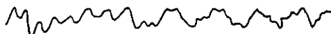
Figure 2. A typical profile of mild steel specimen after surface grinding and polishing.
