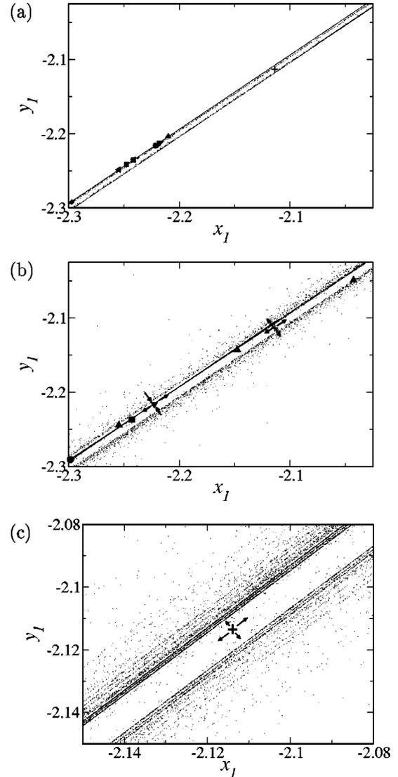
FIG. 4. Poincaré map of system (3): (a)  $d=0.25$ , period-1 UPO (indicated with the cross) is transversally stable; (b)  $d=0.22$ , period-1 UPO (indicated with the cross) is transversally unstable; and (c) enlargement of (b). Also, some low-periodic orbits are shown, which are transversally stable. The location of the Poincaré plane was chosen by setting the base point at some point after sufficiently long integration interval and the normal vector was directed along the flow.
