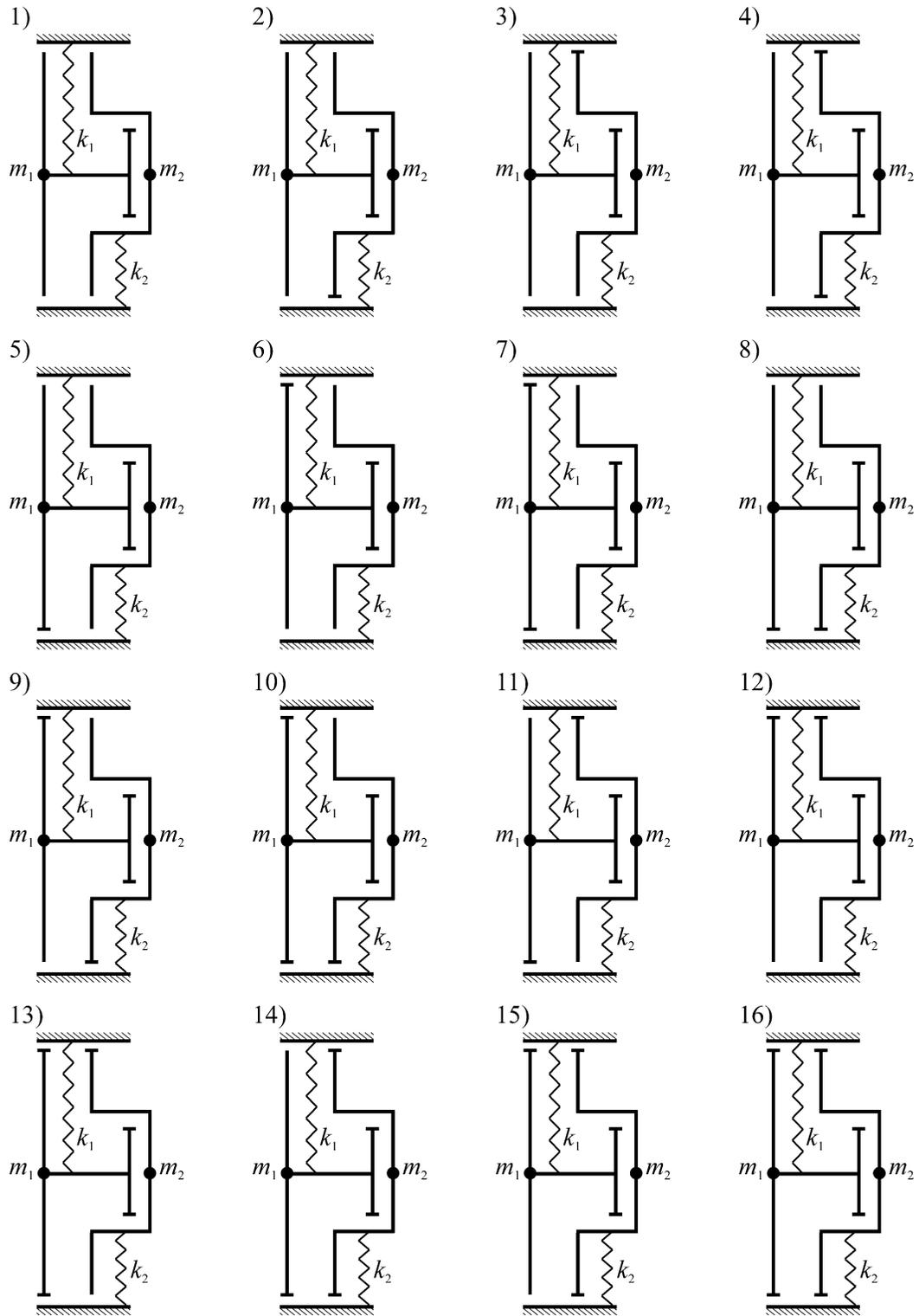
Fig. 13. Possible combinations that arise as a result of the matching of the system with spring combination (8) in Fig. 8 with the systems with fender combinations (1)–(16) in Fig. 9.
