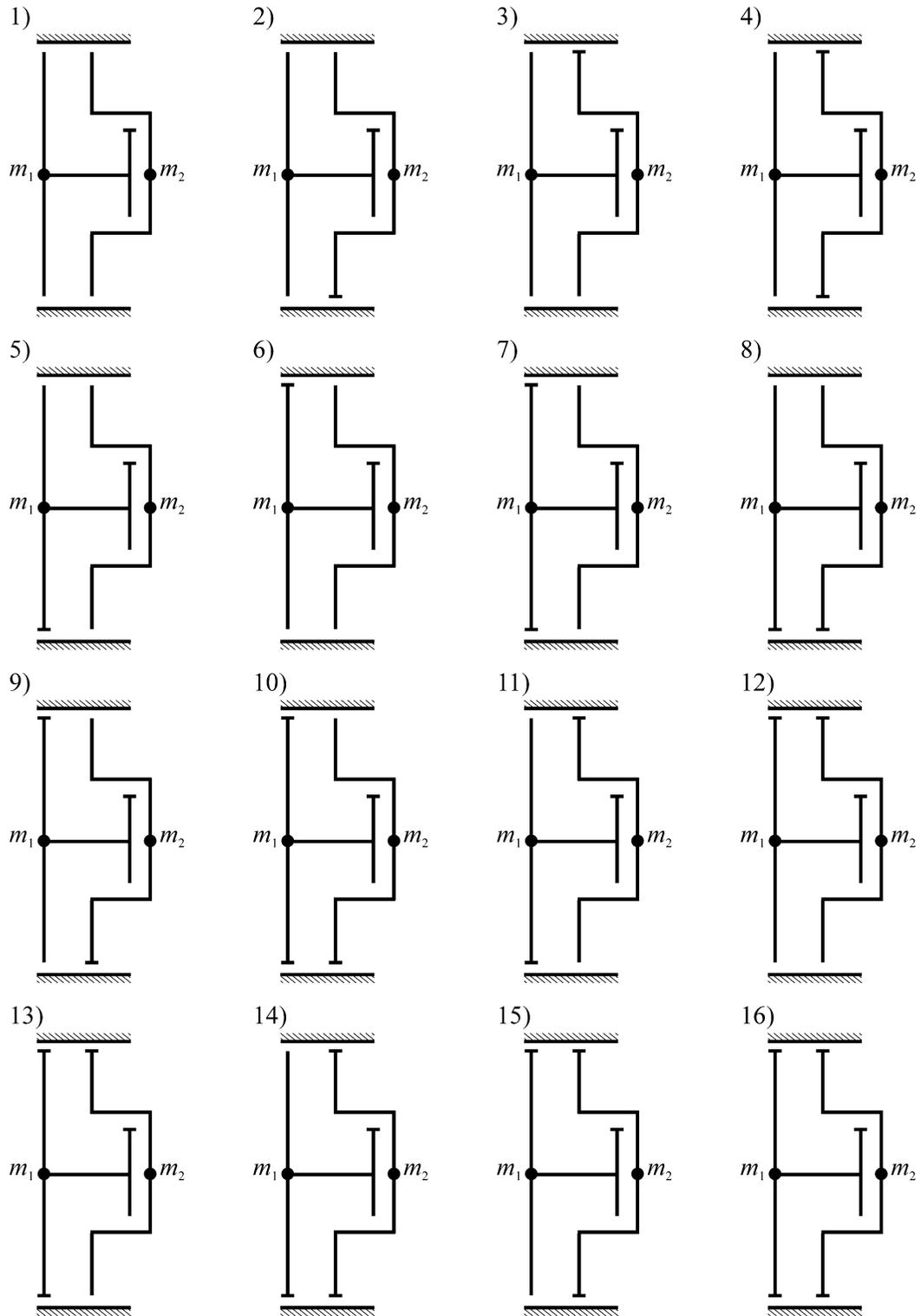
Fig. 10. Possible fender combinations that arise from the basic impact system for  $n = 2$ , including the impact aptness zone (fender  $z_{12g}$ ).
