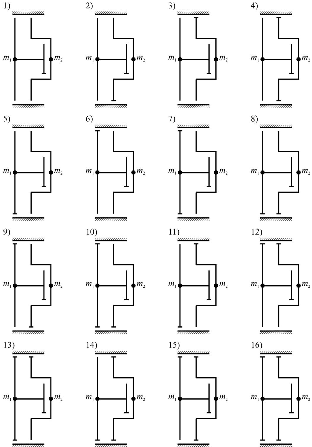
Fig. 11. Possible fender combinations that arise from the basic impact system for  $n = 2$ , including the impact aptness zone (fender  $z_{12d}$ ).
