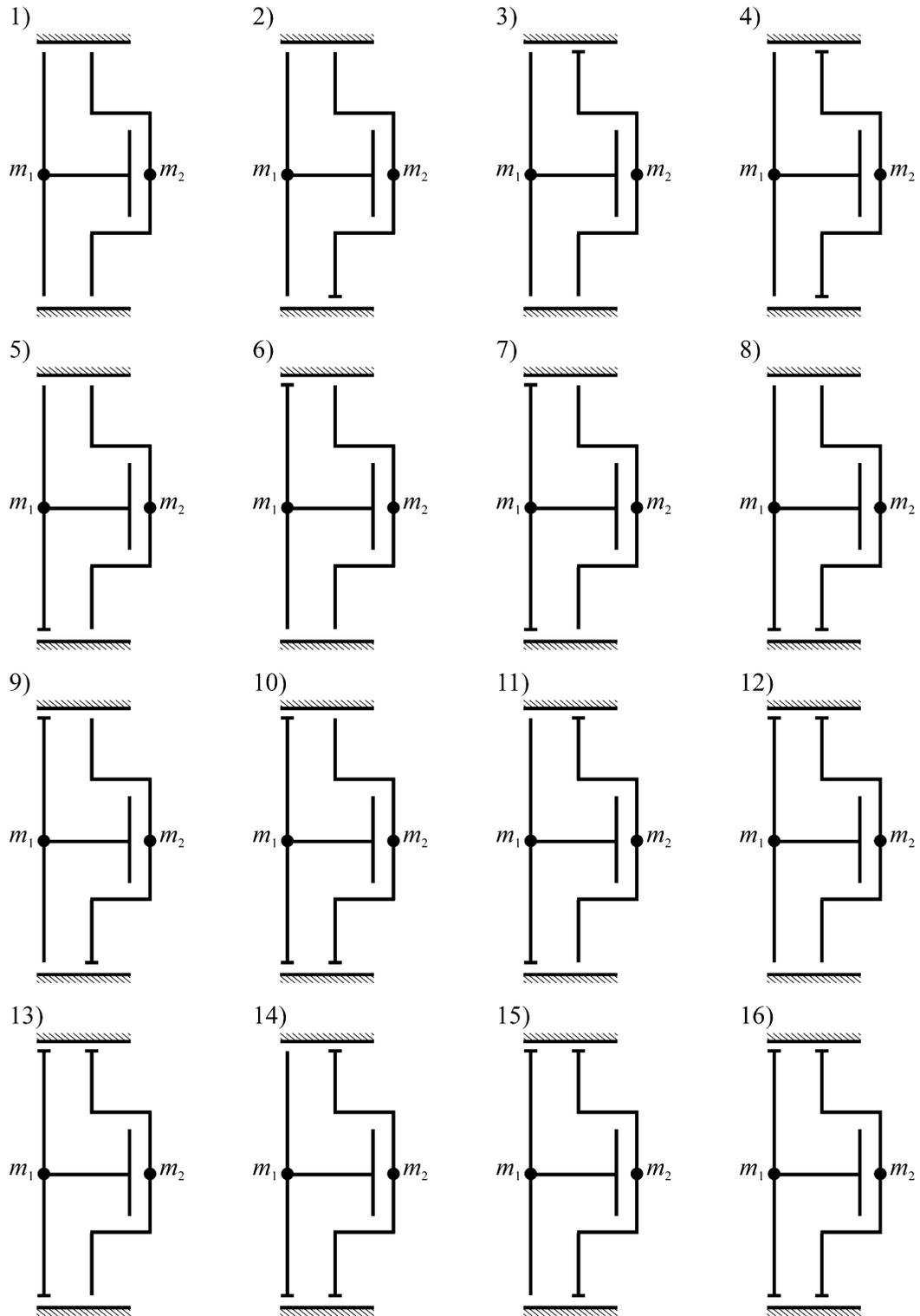
Fig. 12. Possible fender combinations that arise from the basic impact system for  $n = 2$ , without the impact aptness zone.
