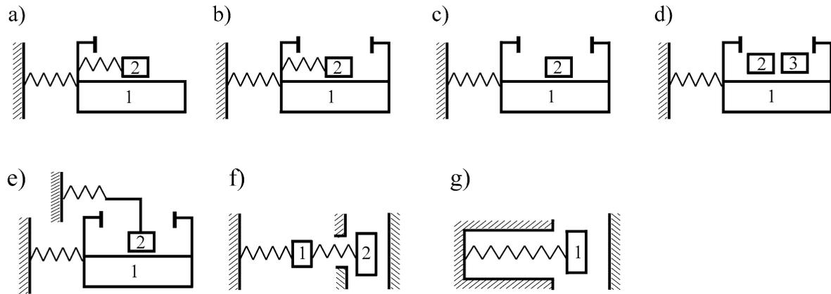
Fig. 1. Schemes of various types of impact vibration dampers.
