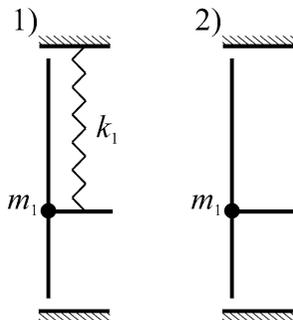
Fig. 14. Possible spring combinations that arise from the basic spring system for  $n = 1$ .
