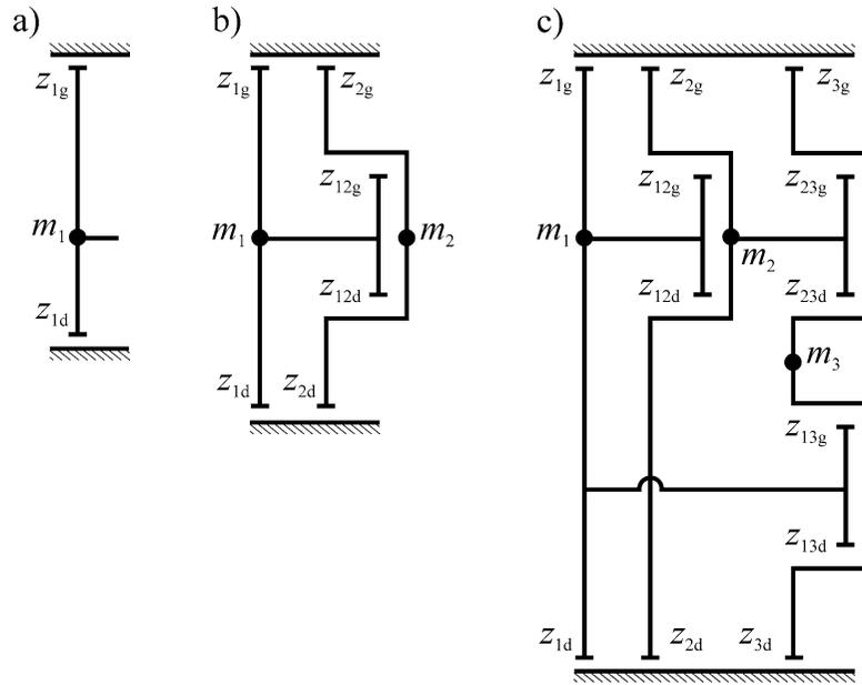
Fig. 5. Basic impact systems: (a)  $n = 1$ , (b)  $n = 3$ , (c)  $n = 3$ .
