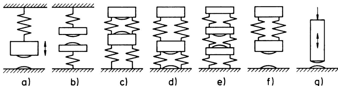
Fig. 2. Schemes of different types of structures in the devices for vibro-impact machining (Peterka, 1981).
