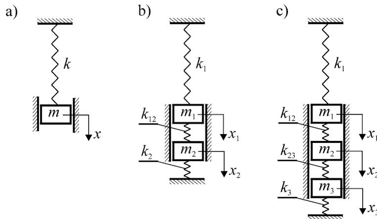
Fig. 3. Schemes of mechanical systems: (a) basic spring system for  $n = 1$ , (b) basic spring system for  $n = 2$ , (c) system with  $n = 3$  that is not the basic spring system.
