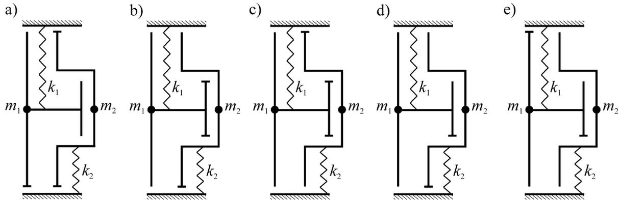
Fig. 7. Examples of the spring–impact combinations for  $n = 2$ : (a) inapt combination in which the basic spring–impact system is divided into two subsystems, (b) and (c) cases identical due to the symmetry of the systems, (d) and (e) cases identical due to the symmetry of the systems after changes in the numbers referring to individual subsystems.
