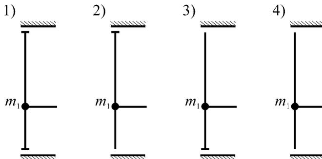
Fig. 15. Possible fender combinations that arise from the basic impact system for  $n = 1$ .
