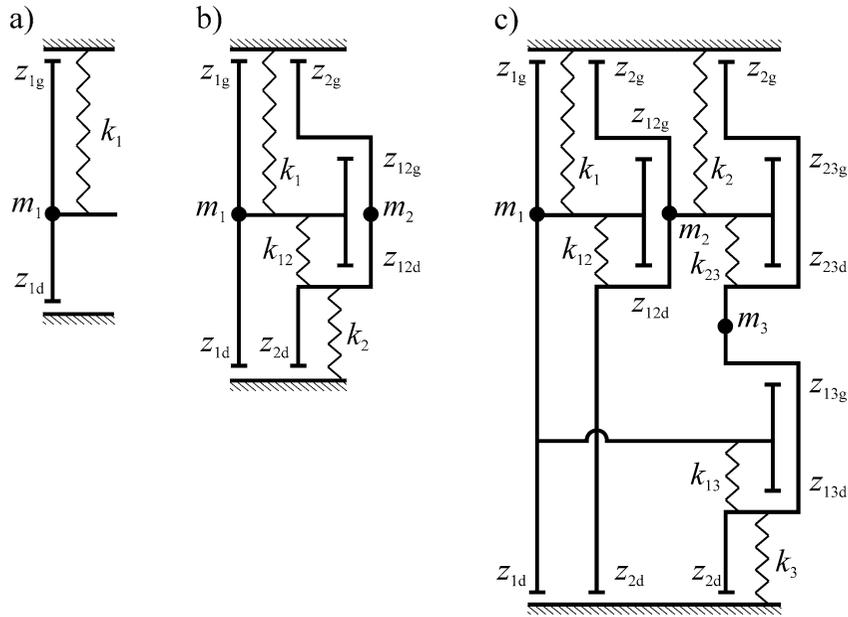
Fig. 6. Basic spring–impact systems: (a)  $n = 1$ , (b)  $n = 3$ , (c)  $n = 3$ .
