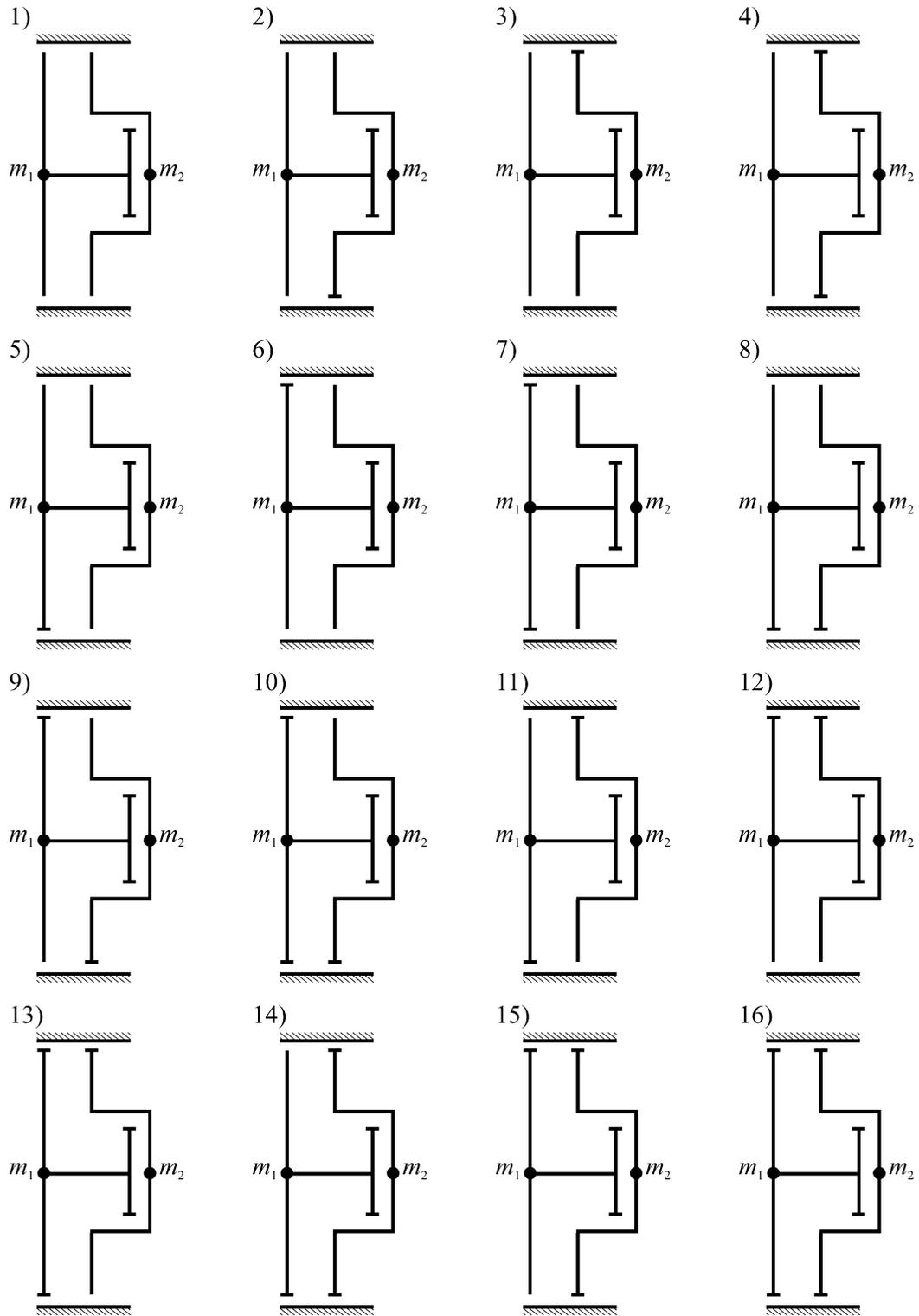
Fig. 9. Possible fender combinations that arise from the basic impact system for  $n = 2$ , including the impact aptness zone (two fenders  $z_{12g}$  and  $z_{12d}$ ).
