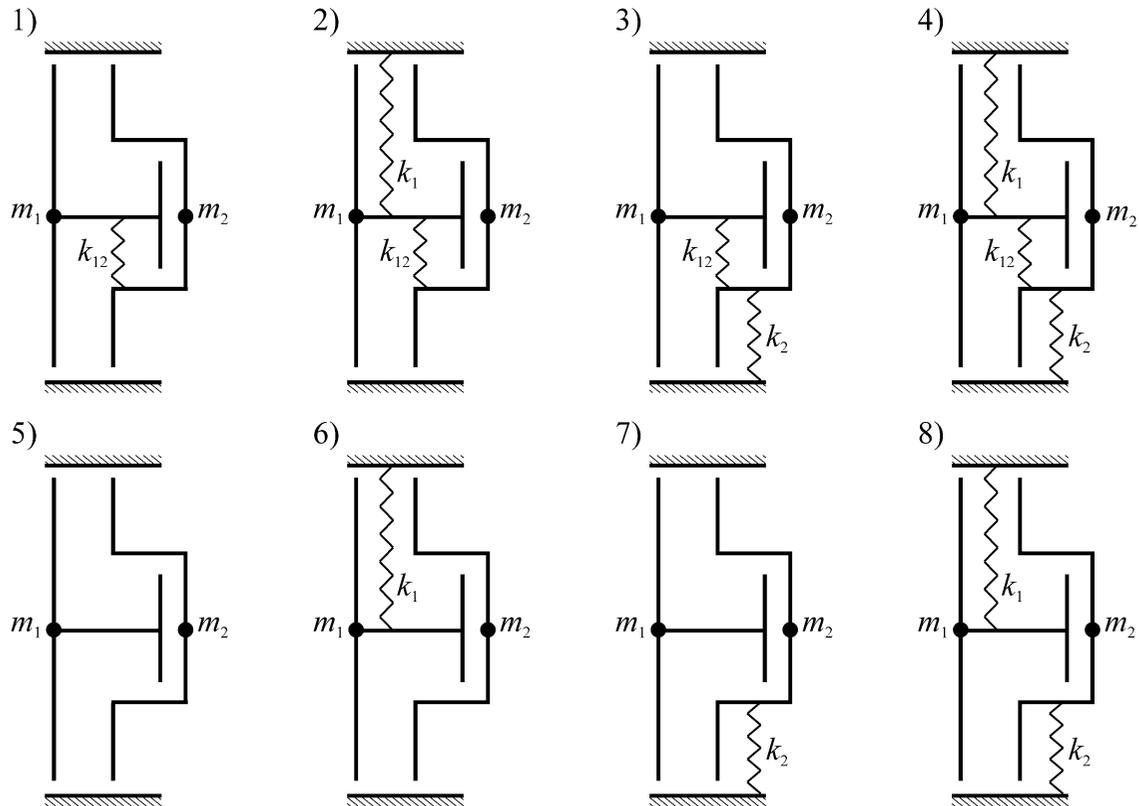
Fig. 8. Possible spring combinations that arise from the basic spring system for  $n = 2$ ; (1)–(4) with the spring aptness zone (spring  $k_{12}$ ), (5)–(8) – without the spring aptness zone.
