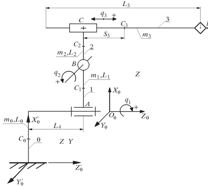
Fig. 14. Scheme of the robot manipulator MAR
