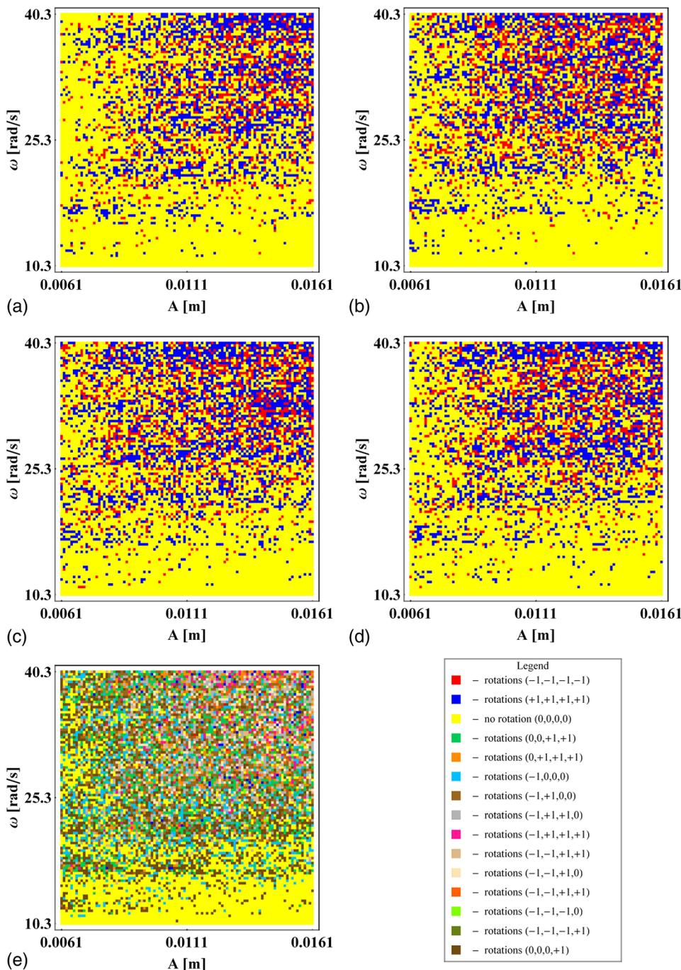
FIG. 4. Different types of pendula’s behavior on the  $A$ - $\omega$  plane (a) pendulum  $II_1$ , (b) pendulum  $II_2$ , (c) pendulum  $II_3$ , (d) pendulum  $II_4$ , red—pendulum rotates clockwise, navy blue—pendulum rotates counterclockwise, yellow—pendulum at rest, (e) combined synchronous states of 4 pendula.
